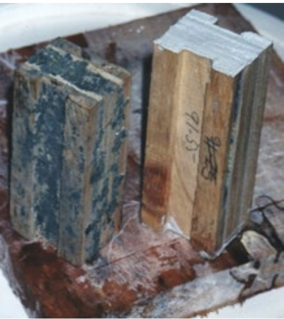
Mold trial: untreated — left, treated — right.
