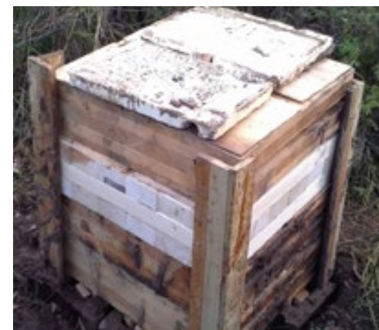
CLT termite trial.
