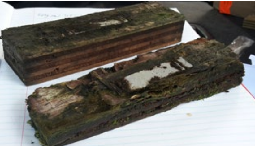
Plywood in a trial in Hawaii: treated top, untreated bottom.
