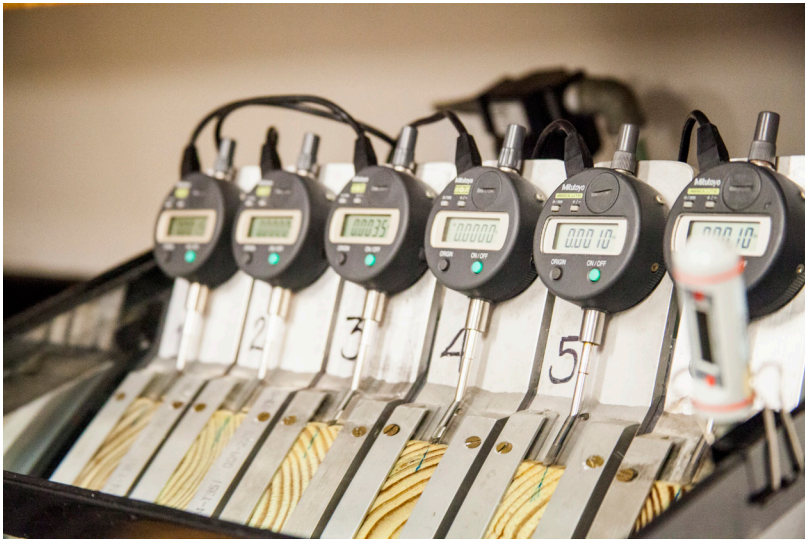
American Wood Protection Standard E13-09 was established in 1992 to test the water repellency of wood. The Swellometer above is used for the testing.
