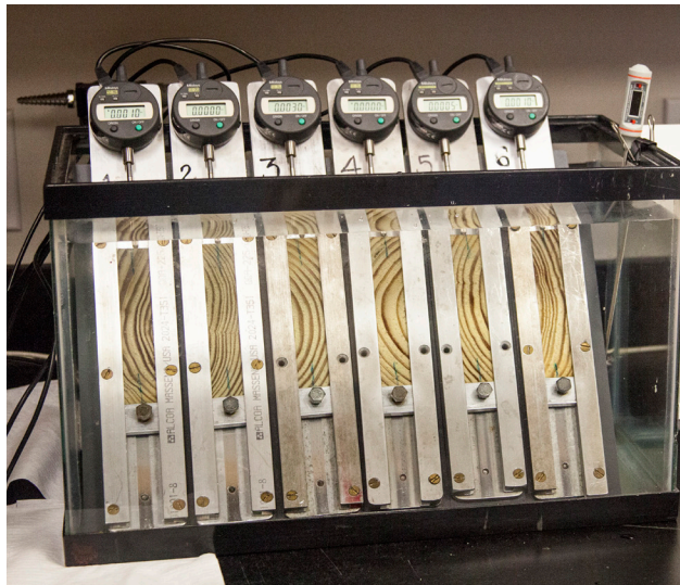
American Wood Protection Standard E13-09 was established in 1992 to test the water repellency of wood. The Swellometer above is used for the testing.
