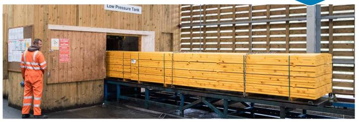
Vacsol low pressure treatment facility (photo courtesy of BSW Timber).
